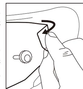
7 To make the CWR-F2R tear-off film easier to remove, gently fold the slightly longer part of its front right edge toward you.
