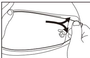
4 Peel off only the protective sheet on the side of the CWR-F2R tear-off film that will adhere to the shield/visor and then attach the film starting from the left CWR-F2R tear-off button with reference to the shield/visor. After this, adhere the CWR-F2R tear-off film while lightly pulling it toward the right.
