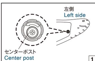
Turn the main part of the CWR-F2R tear-off buttons attached to the CWR-F2R shield/visor counterclockwise and adjust them so that their center post is at the bottom when the shield/visor is viewed from the front as shown in Drawing 1.
