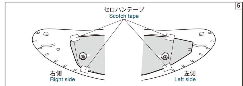
6 Cut scotch tape into 15 mm x 20 mm slits and stick them on locations indicated in Drawing 5.
