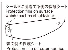
3 After adjusting the tension, detach the CWR-F2R tear-off film from the shield/visor and once again remove any dust or oil adhered to the surface of the shield/visor.
