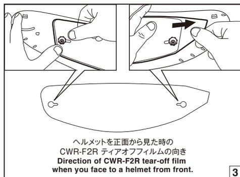
1 First, remove any dust or oil adhered to the surface of the shield/visor. Next, check the left/right direction of the CWR-F2R tear-off film and, with the protective sheets still attached to both sides, mount the film on the CWR-F2R tear-off buttons as shown in Drawing 3. At this time, check the CWR-F2R tear-off film is securely attached to the surface of the shield/visor.
