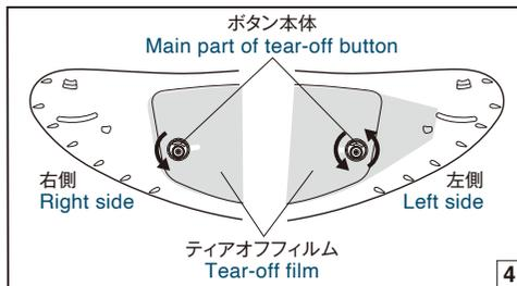
2 If the CWR-F2R tear-off film is not adequately attached, turn the left and right buttons counterclockwise (Drawing 4) to increase the tension of the film and properly secure it to the shield/visor.
