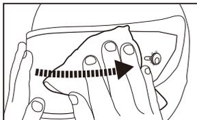
5 Securely attach the CWR-F2R tear-off film to the shield/visor while using a towel, etc. to push out any air bubbles between the two surfaces. Next, remove the protective sheet on the front surface.
